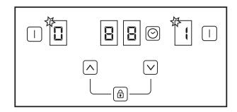
**3.** After a few seconds all symbols will disappear on the zone display and an audible alarm will sound and return to standby mode.
