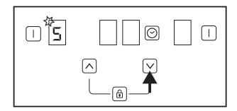
The relevant cooking zone will start to operate at the set temperature level.
