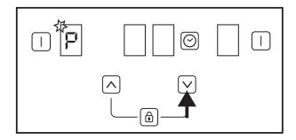
Selected cooking zone will operate with maximum power "P" symbol will appear on the cooking zone display. Cooking zone will switch itself off when the booster time is up.
