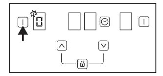
The hob will automatically return to standby mode if no operation is performed within 10 seconds.
