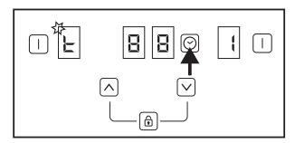
**4.** Adjust the desired cooking time by touching  $\checkmark$  keys.
