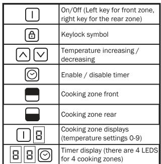
During the initial start up of the hob (or power failures)  $\begin{bmatrix} \mathbf{B} \end{bmatrix} \begin{bmatrix} \mathbf{B} \end{bmatrix}$  will be displayed for several seconds and an audible alarm will sound.
