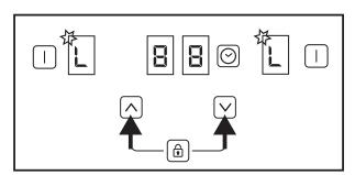
Only one signal sound will be heard. Key lock function is activated and "L" appears on all cooking zone displays.
